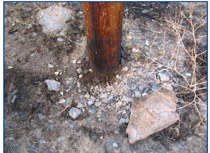
Close-up of the pole that shocked the Engine Boss. Notice the burned creosote and charring on pole. The Engine Boss's footprints can be seen in the lower left of image. This is where he was located when the electrical shock occurred.
